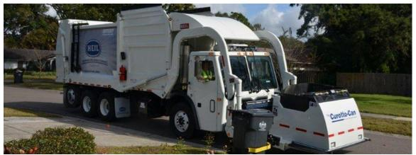
Figure 1. Heil Odyssey AFL with integrated Curotto-Can
