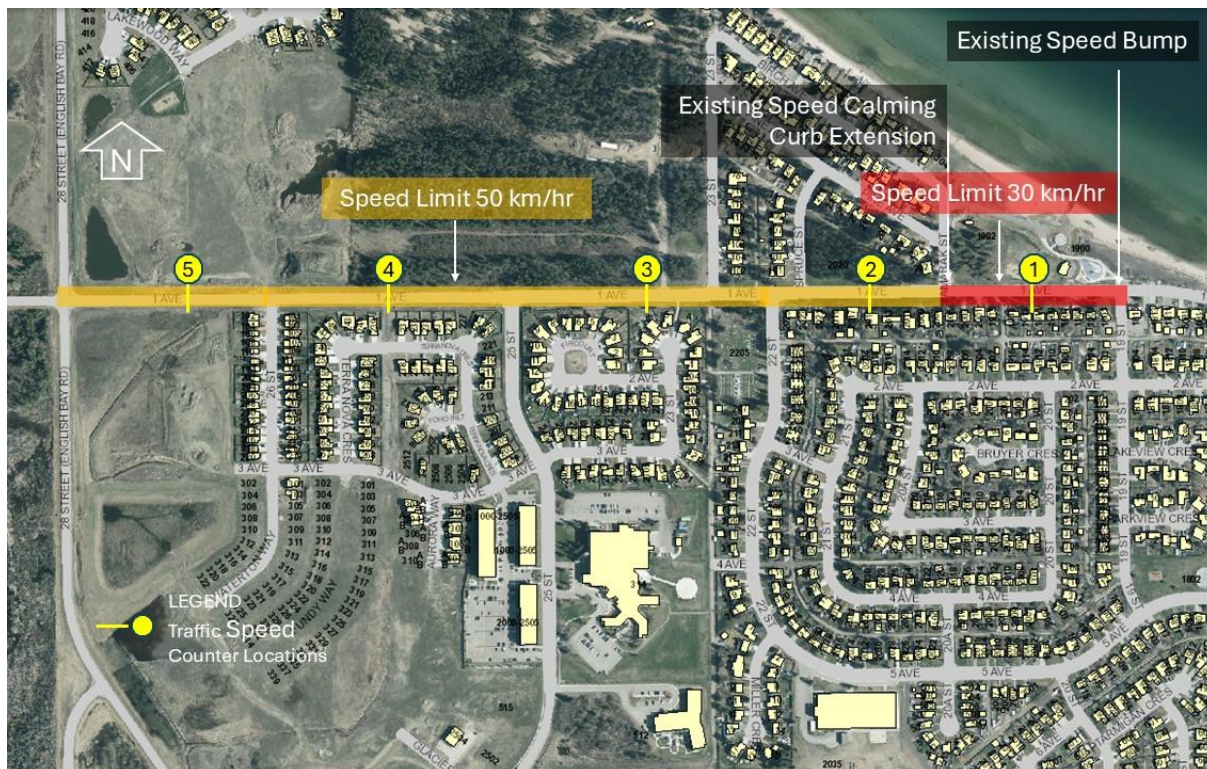
Figure 2. Overview of location and extent of speed limit zone, and location of speed counters on 1 Avenue between 19 St and 28 St
